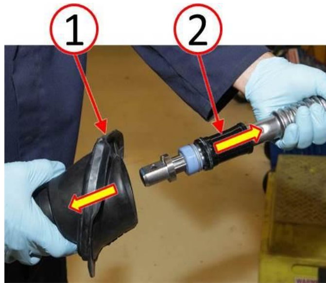
Fig. 2 Remove Boot From Intermediate Shaft
