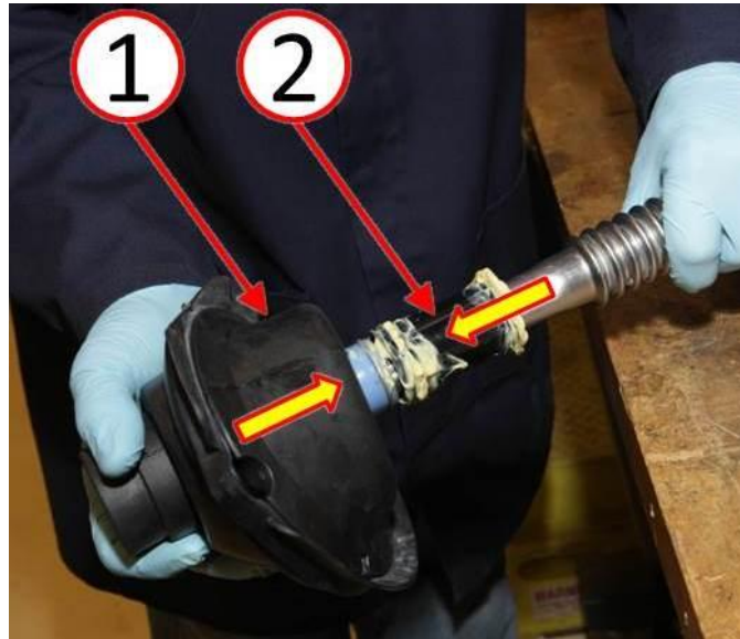
Fig. 8 Install Boot To Intermediate Shaft
