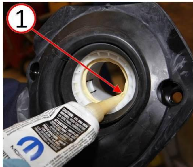
Fig. 7 Apply White Lithium To Outer Bearing Sleeve
