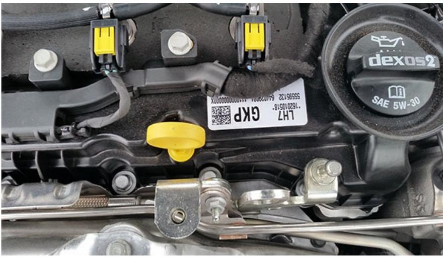
As shown in the above photo, the engine broadcast code can be found on the engine valve cover.
