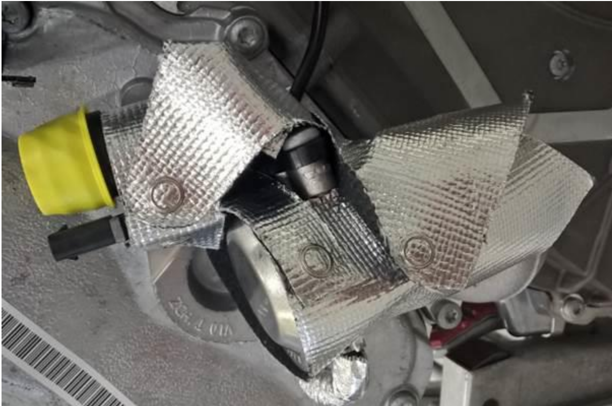
Figure 2. Insulation on Bank 2 pressure sensor after installation.
