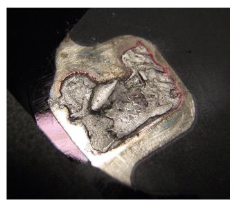
3. Prepare the surface of the used defroster tab (not required for new tabs on new-style full-size utility models) and the defroster buss bar with fine grain (500 grit) sandpaper or Emery cloth. It is not necessary to remove all of the original solder, but it should be scuffed sufficiently so that no oxidation is present. The photo above shows a close up of a properly prepared surface.
