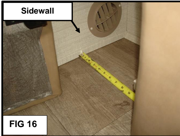
FIG 16: Left side sofa roller: Locate the right side edge of the right side mounting bracket. Measure from the side wall as shown, under the sofa to the bracket edge.
