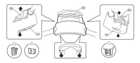
• After disconnecting all the wiring harness connectors, **CAREFULLY** remove the roll connector, steering angle sensor and the combination switch assemblies. **IMPORTANT:** Do not disturb the postion of the roll connector while removed from the steering column. As shown in the photo, use a piece of tape to keep it in alignment while removed.
