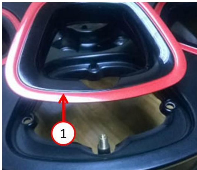
Fig. 3 Place insert onto front of wheel
