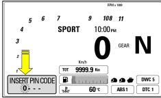
2) using the UP and DOWN buttons of the left-hand switch it is possible to enter the Pin Code set by the Customer and start the engine.
