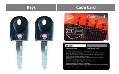
The **black keys** contain the electronic device (transponder) that allows starting the engine only if the same key is acknowledged by the instrument panel control unit.
