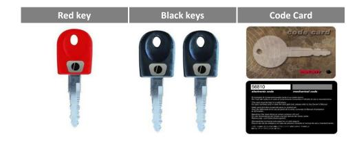
The **Red Key**, also called "Master Key", allows starting the engine and is the only one that allows programming, deleting and reprogramming the black keys.
