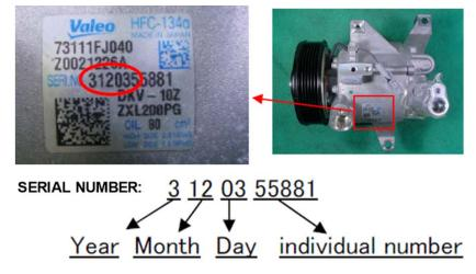
• If the Serial Number is **50930**\*\*\*\*\* or **BEFORE** (September 30, 2015), replace the A/C compressor assembly following the procedure outlined in the applicable Service Manual.
