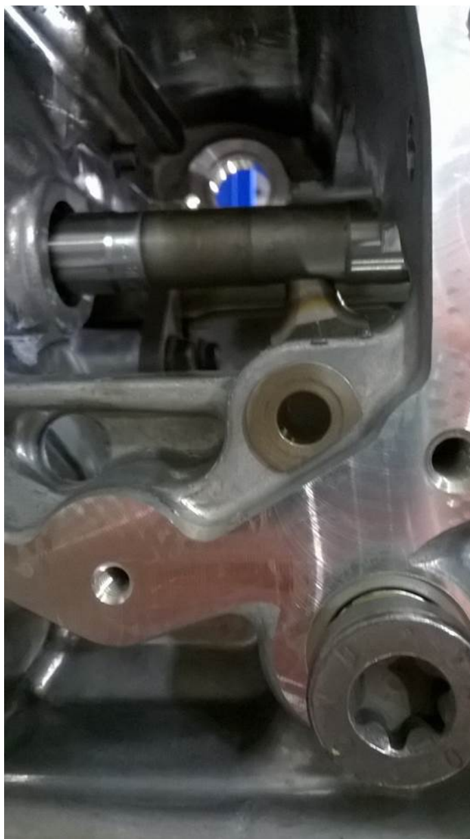
Figure 2 – New Steel Bushing Installed
