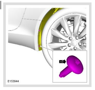
Remove the rear wheel arch liner fasteners.
