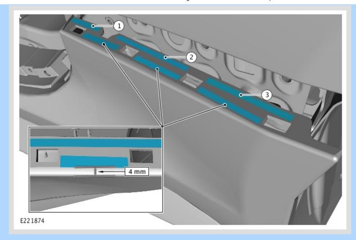
Install the adhesive tape to the areas of contact.
