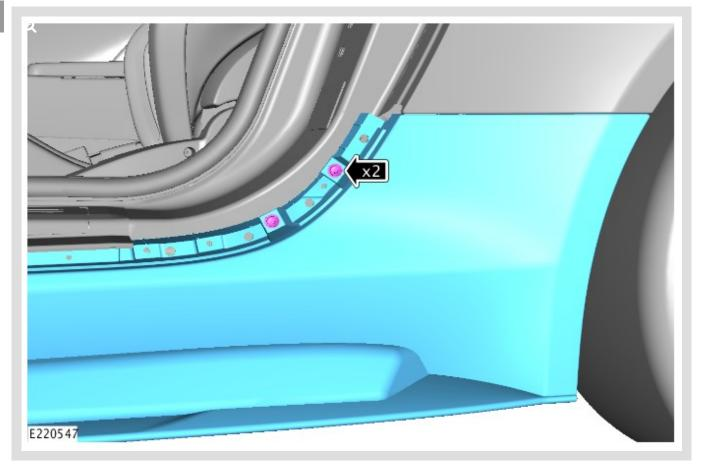
Remove the fasteners.
