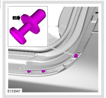
Remove the fasteners.
