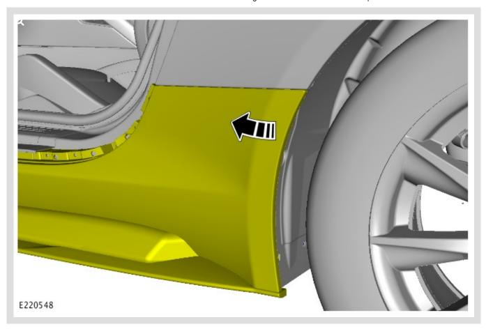
Position the rocker panel moulding to one side.
