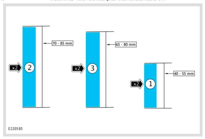
Cut the adhesive tape to the sizes and quantities shown.
