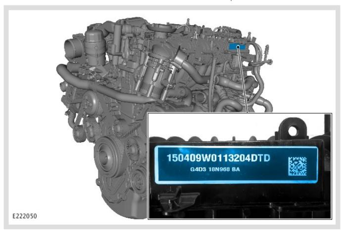
Locate and record the engine serial number.
