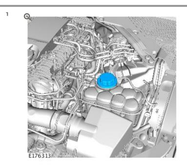
Remove the engine coolant expansion tank pressure cap.
