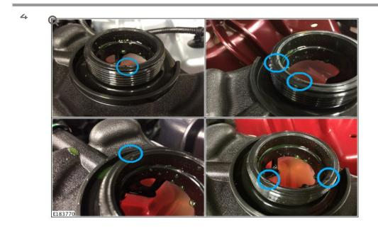
Visually inspect the sealing bead on the engine coolant expansion tank neck to check for damage.
