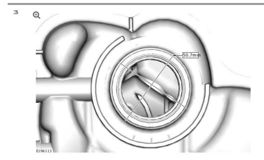
Check the dimensions of the engine coolant expansion tank threaded neck in the two positions shown.
