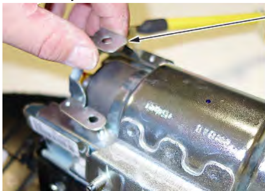
INFLATOR BRACKET Do not reuse.
