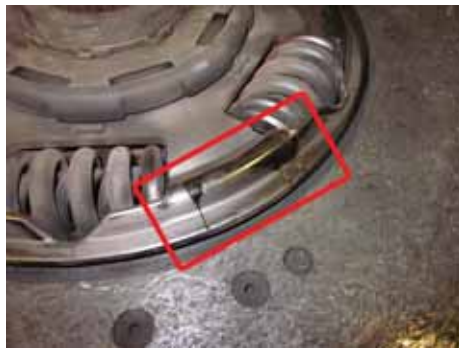
Engine Oil Accumulation in Bottom of Flywheel Housing
