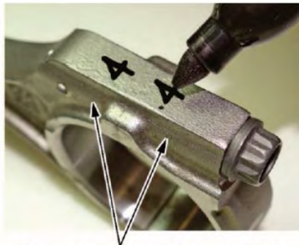
Mark the connecting rod and rod cap with the cylinder number.
