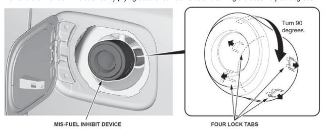
2. Tilt the mis-fuel inhibit device towards the rear of the vehicle to remove it from the fuel fill pipe.
