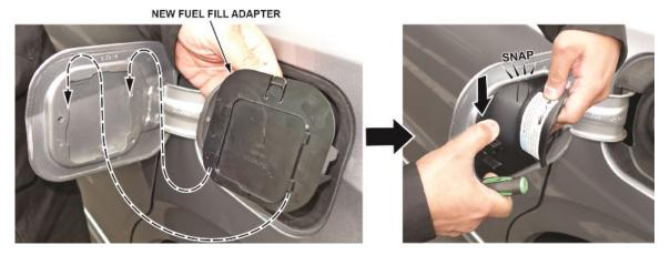
7. Make sure the fuel door closes and latches without contact or interference from the mis-fuel inhibit device and surrounding area. The gap between the door and the surrounding quarter panel should remain consistent.
