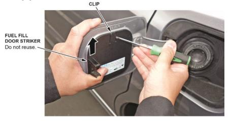
6. Installation of the fuel filler lid striker is the reverse of removal. Verify all the tabs are engaged, and slide the lid downwards until it clicks. This indicates the fuel filler lid striker is secured and correctly installed.
