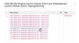
**If software is current and the code is present,** the code confirmed status should be verified to be True as shown above before continuing diagnosis. If the status is False and there are no related codes or symptoms, clear the code and release the vehicle.
