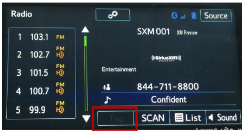
U.S specification: Tag button is outlined and either selectable or grayed out (as shown).
