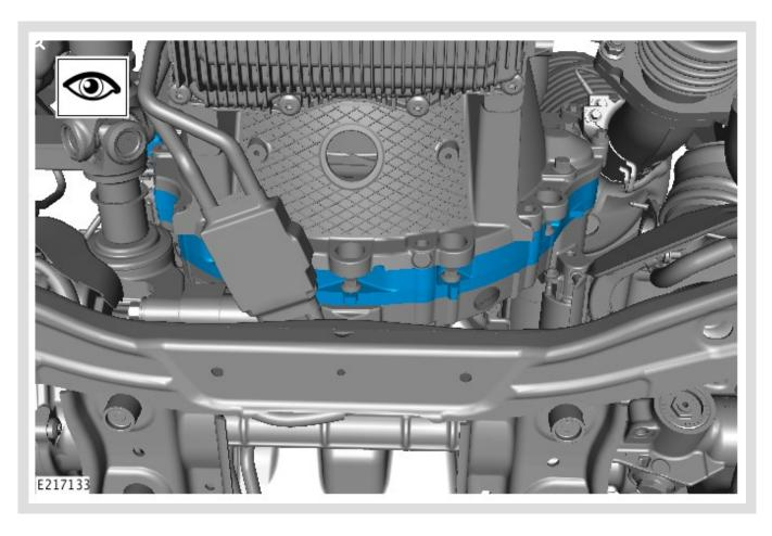
Inspect the engine lower timing cover area for an oil leak.
