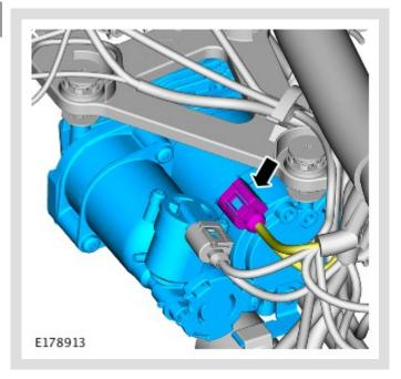
Location of the air suspension compressor electrical connector to be replaced.
