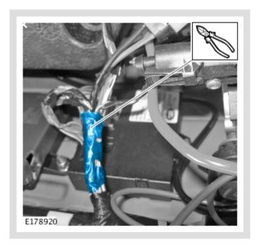
Use a suitable tool to remove the securing tape from the electrical wiring harness.
