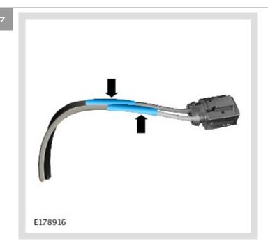
Install the new electrical connector to the original electrical wiring harness (see TOPIx Workshop Manual section 418-02: Wiring Harnesses).
