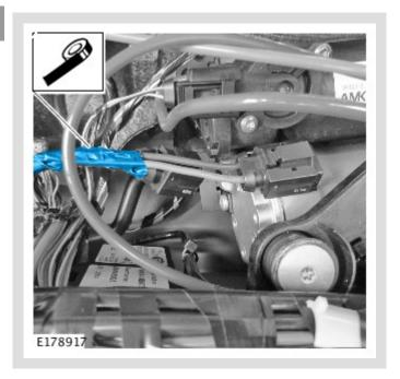
Use a suitable tape to secure the electrical wiring harness in the area shown.
