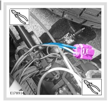
Cut the electrical connector in the area shown. Make sure the electrical wiring harness is cut in a staggered position.
