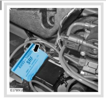
Install the electrical wiring harness label.
