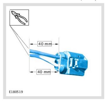
Cut the new electrical connector off the new electrical wiring harness.
