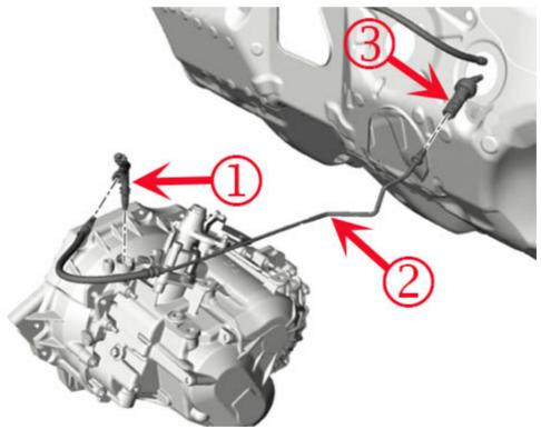
The source of the debris is the dampener in the high pressure line (3).
