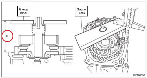
5) Obtain the thickness of transfer driven gear shim using the following formula to select zero to three transfer driven gear shims.
