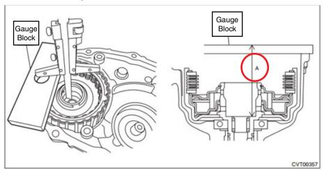
4) Using the Gauge Block, measure the height "B" from the transmission case mating surface to the end of the Gauge Block
