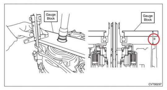
4) Obtain the thickness of reduction driven gear shim using the following formula to select zero to three reduction driven gear shims.
