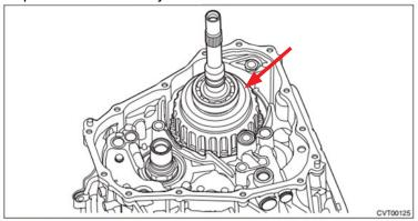
2) Measure the height "A" from the Gauge Block upper face to the ball bearing catch surface.
