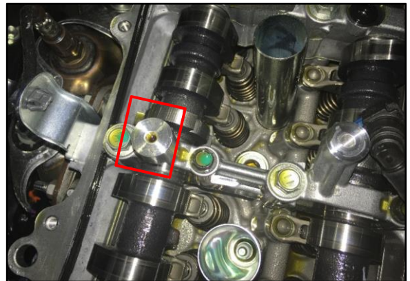
Figure 4. Cam Sensor Bolt Hole (Valve Cover Removed)
