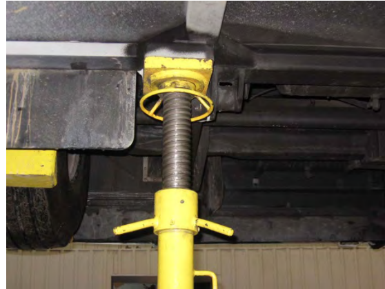
FIGURE 4 : JACK STAND AT CHASSIS HOISTING POINT - AFT OF FRONT AXLE (BOTH SIDES)
