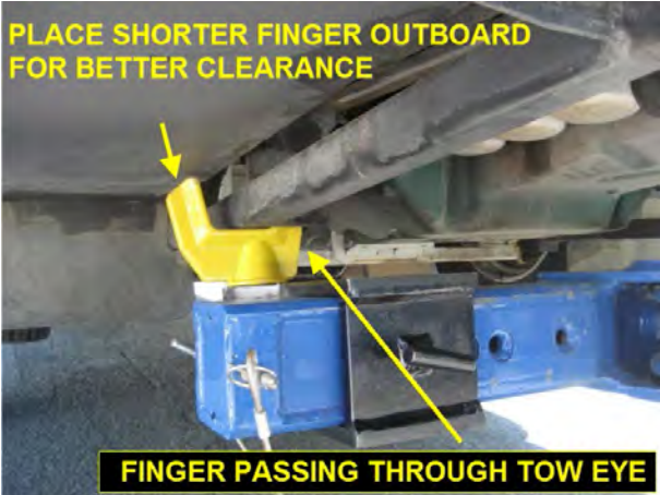
FIGURE 62 : PROPER LOCATION WHEN LIFTING THE SIDE MEMBERS – VEHICLE EQUIPPED WITH REAR TOW EYES
