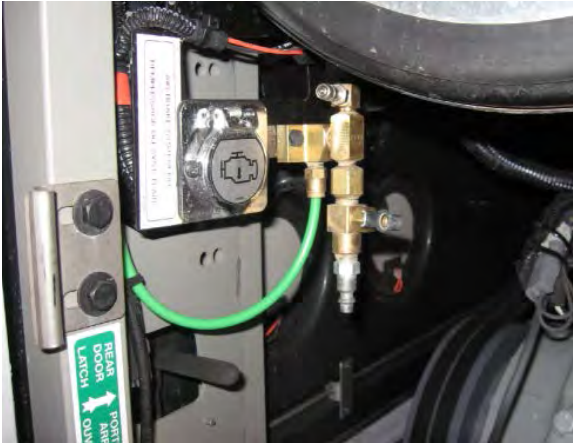
FIGURE 23 : ENGINE COMPARTMENT EMERGENCY AIR-FILL VALVE
