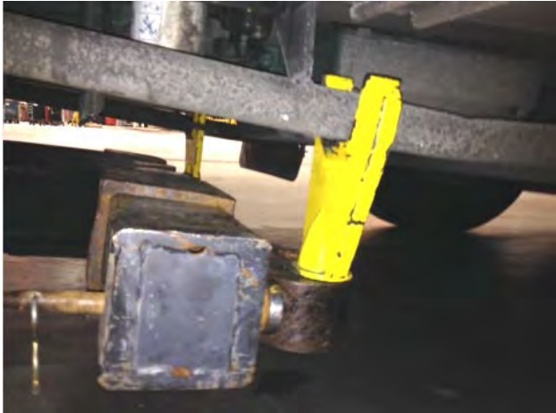
FIGURE 61 : PROPER LOCATION WHEN LIFTING THE SIDE MEMBERS
