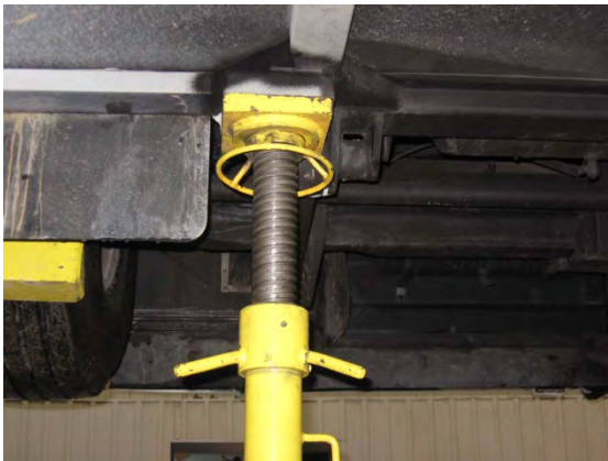
FIGURE 17 : JACK STAND AT CHASSIS HOISTING RECEPTACLE - AFT OF FRONT AXLE, ROAD SIDE
