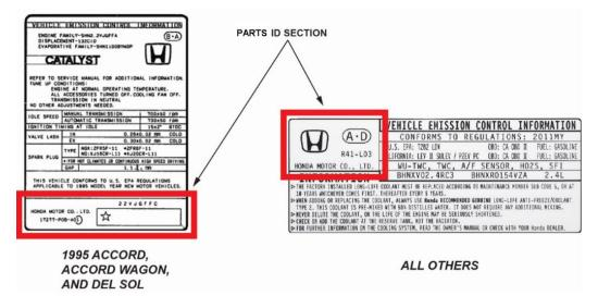
4. **1995 Accord, Accord Wagon, and Del Sol only:** Compare the part number on the label to the part number in the table below:
