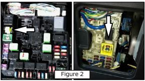
During shipping of Mitsubishi vehicles, dark current is minimized by not connecting the IOD connector. It is positioned in the disconnected position (pulled up) and must be connected by pressing it down for the affected circuits to be completed.
