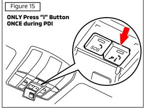
19. <u>Perform test of Mitsubishi Connect System</u> (Eclipse Cross models only, if equipped).
