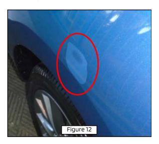
NOTE: If there is still discoloration or blotching or a "milky" color on the paint surface after RAP-Film removal and cleaning (as shown in Figure 12), <u>DO NOT REPAINT THE VEHICLE</u>. Submit a PRC entry with photos for DPSM review, then send the vehicle to a body shop that can use an ultraviolet heat lamp to eliminate milky color spots.
