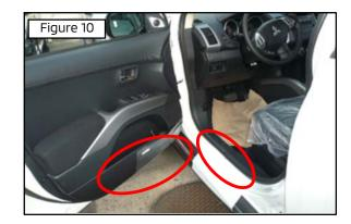
For certain models, the driver entry area is protected by a <u>clear</u> RAP-film placed on the scuff plate and/or lower door area. This is to protect the area from damage while the vehicle is available for viewing by customers or in dealer storage, improving Initial Quality Survey (IQS) scores. The Outlander is protected in both areas and the Lancer is protected on the lower door only.
