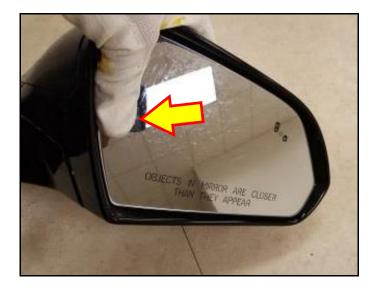
3. Wrap a clean towel around a small flathead screwdriver and carefully pry at the two corners of the mirror to remove it from the assembly.
