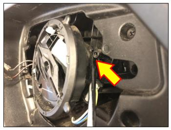
Actuator removed. Image on the right illustrates the position of the three mounting tabs.
