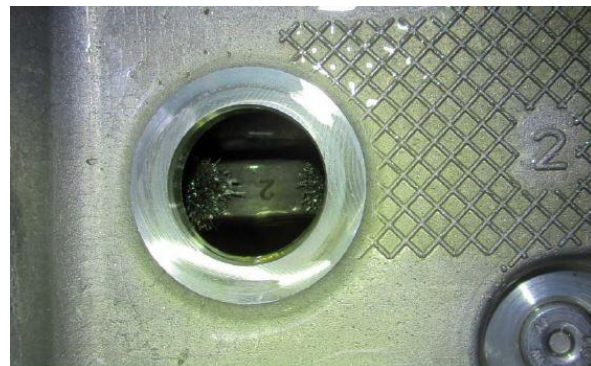
Figure 3. Selector magnet for gear actuator 2/6.
