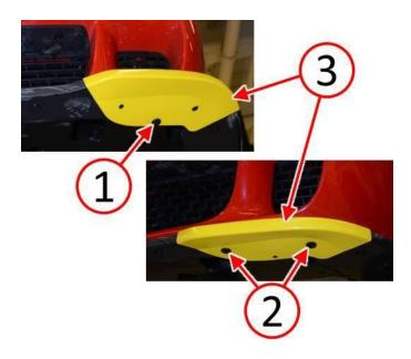
Fig. 2 Remove Front Air Dam Shipping Covers
