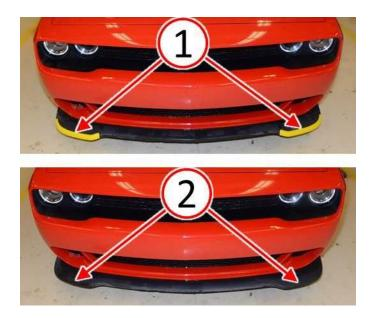
Fig. 1 Inspect Front Air Dam For Shipping Covers
