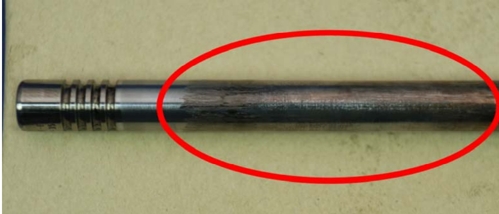
Figure 2 Valve Stem With Visible Wear
