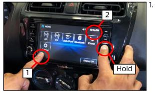
While pressing the "Home" button, touch the bottom left corner of the Audio Display briefly. Then touch the top right corner of the Audio Display for at least 2 seconds.
