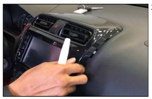
2. Use an ornament remover to remove the instrument center panel.
