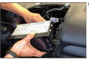
5. While removing the Display Audio component, disconnect the radio antenna, the radio/CD player harness, and two connectors (20-pin and 8-pin).
