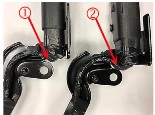
Before installing a new jumper harness be sure to inspect the wiring harness. As seen above 1. shows a good harness 2. shows a suspect harness. if the harness looks like number 2 please adjust the harness as needed.
