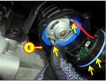
12. Slowly rotate the cap (F) a half-turn counterclockwise to cross the wires and push firmly until the cap is completely seated to the vacuum pump.
