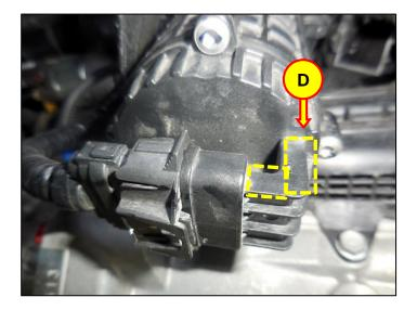
4b. Apply (2) coats of sealant on both sides (D).
