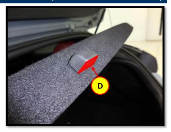
3. Insert the new damper (C) to the covering shelf (B). Pull the damper to clip against the covering shelf using a plier or a similar hand tool.
