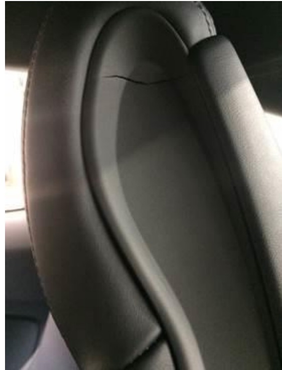
Figure 3. Front seat side trim cracked.
