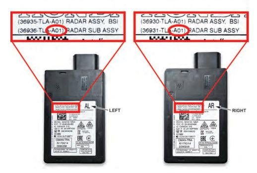
A replacement BSI radar unit should be replaced only with one that has the exact same part number. When replacing the unit, make sure that the last three digits of the part number, A01 or A02, are matching on both sides. Even though these units look the same, the parts can't be interchanged without causing problems in the software, which will result in the applicable DTC (B18DA or B1EDA) to set.
