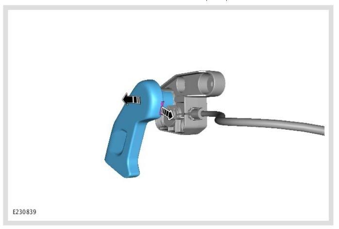
Remove hood interior release lever from the hood release mechanism.
