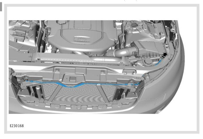
Remove the hood release cable from the vehicle.
