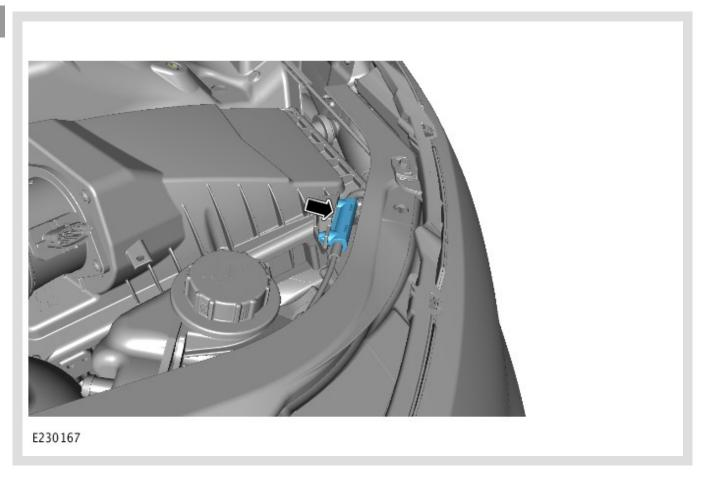
Release the hood release cable from the retainer.
