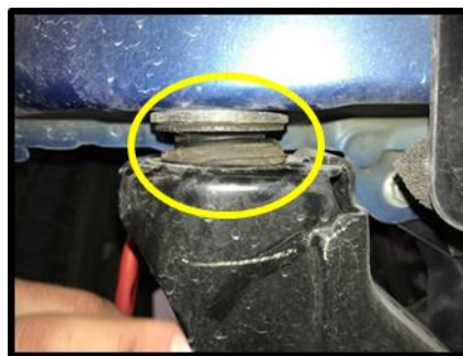
Example of bushing condition photo
