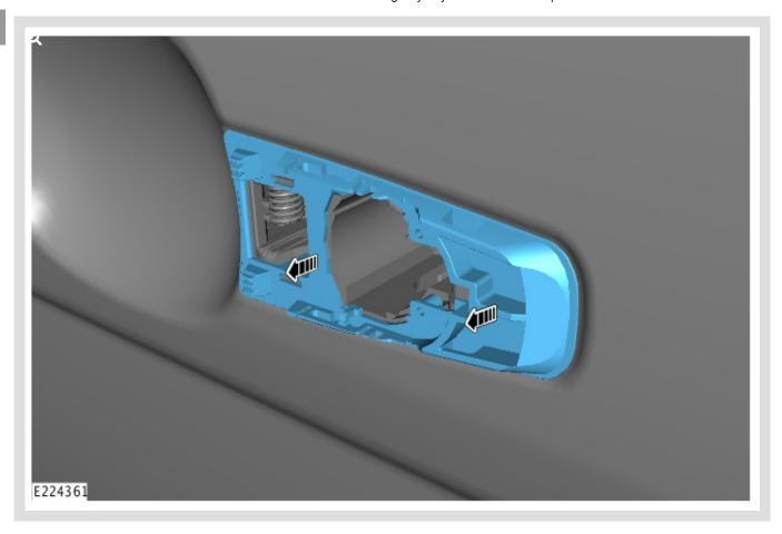
Remove the front left door exterior handle gasket.
