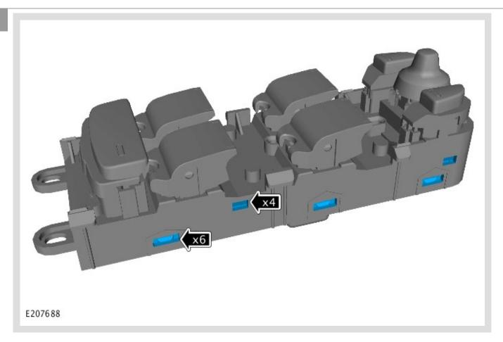
Apply sealing tape to both sides of the **new** driver door (master) window switchpack, covering the side cavities on the driver door switchpack.
