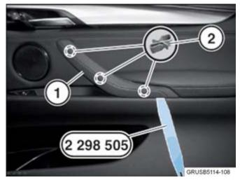
4. The latching mechanisms (1) of the cover (2) must not be damaged.
