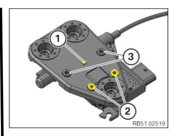
16. Replacement: Remove the lug (1) and grind the lugs (2) to the same height as the lugs (3).
