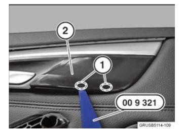
6. Pry the catches in area (1) using special tool 00 9 321. Unclip the trim (2).
