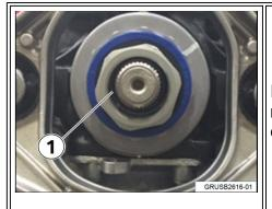
Identifying the 8 090 464 differential: Check the number of splines on the old/new differential. **The correct differential has 35 splines (1)**
