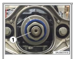
Identifying the 8 090 473 differential: Check the number of splines on the old/new differential. **The correct differential has 27 splines (1)**
