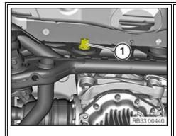
During the repair, when releasing rear differential Hexagonal collar bolt M14x1.5x125 (PN 33 17 7 852 488), make sure that the bolt's hex head does not show any marks indicating previous removal. In case bolt M14x1.5x125 (1) has been removed (torque released) previously, it needs to be replaced together with 4 sub-frame Torx screws M12x60 (PN 33 30 2 284 642).
