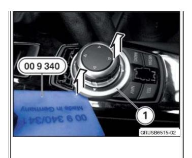
2. Carefully pry the chrome ring from the controller latch mechanism with special tool 00 9 340. Remove upwards.
