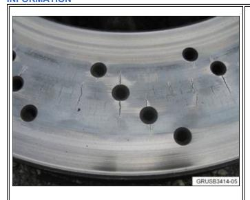
1. Visible cracks are caused by high thermal stresses during rapid heating and cooling of the brake discs. Braking from high speed with cold brake components (less than 212 degrees F) increases the likelihood of cracks to form. These surface hairline cracks are usually spread over the entire brake disc friction area, and have no negative influence on the durability or braking performance. The rotors should not be replaced only for their appearance reasons.
