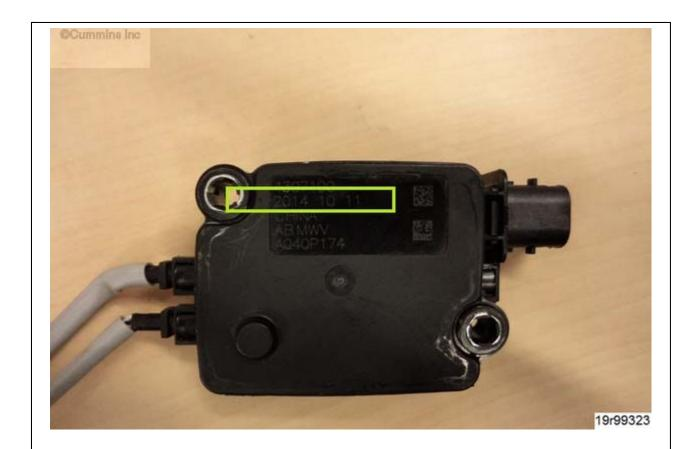
Figure 1, Date Code Location on the Aftertreatment Exhaust Gas Temperature Sensor.
