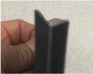
Both doors CAN have the overmold seal cut back as shown. However one should be sufficient.
