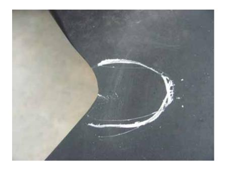
${f 2.}$  Grind or prepare the marked areas: Ensure good adhesion by using a burr bit to grind out the crack on both the top and bottom surfaces.
