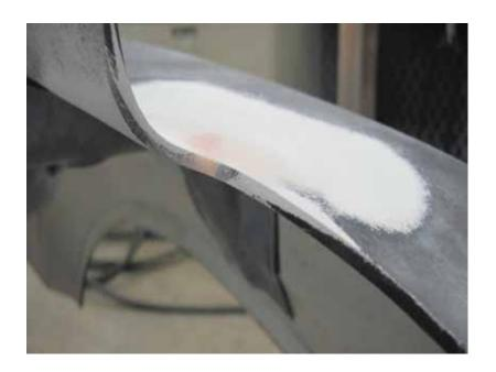
8. Using a clean mixing board and spreader, mix the Metal Glaze and Hardener together thoroughly and cover the areas where Fibral was applied.
