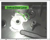
Retrieve & install defrost door lever. Insure that lever 'snaps' into defrost door shaft. Insure that lever is oriented as shown.
