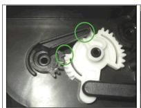
Retrieve & install 2<sup>nd</sup> defrost door lever. Insure that lever 'snaps' into defrost door shaft. Insure that lever is oriented as shown. Insure that lever pin is contained in gearcam track.
