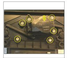
Rotate fixture 180°. Retrieve & install actuator to kinematics sub-assembly. Drive (6) screws to actuator & kinematics sub-assembly.
