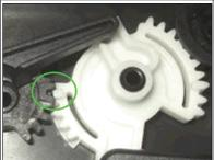
Visually verify that gears were initially properly aligned.
