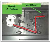
Retrieve kinematics sub-assembly & install to housing as shown. *Insure that lever 'snaps' into vent door shaft.*
