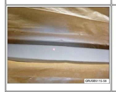
5. Mask off the area of the roof and clip for the roof frame trim strip and apply a preservative to the repaired area.
