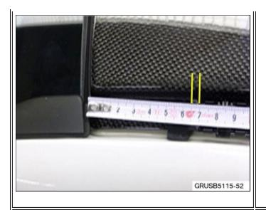
2. Locate the area by the carbon fiber roof panel. The area to be inspected is on the left side approxmately 65 to 69 cm from the front edge.
